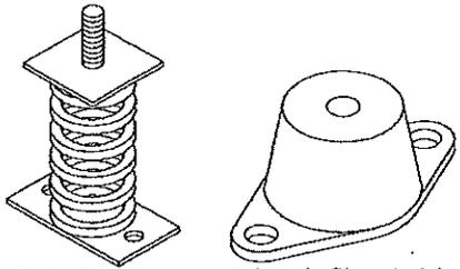
Spring Isolator Rubber-In-Shear Isolator
