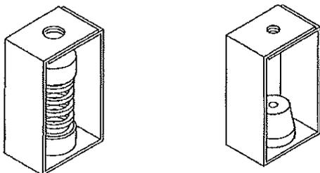
Ceiling Mounted Spring Isolator Rubber-In-Shear Ceiling Isolators
